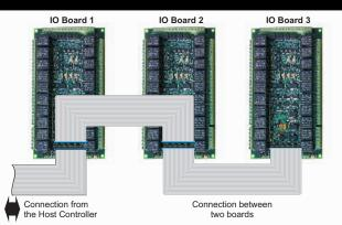
I/O expansion board also known as Input-Output expansion board consists of 20 relays and 8 opto-isolated inputs. It works on 12 VDC supply. Each of the relay consist of three terminals on the board namely N.O. (Normally Open), N.C. (Normally Closed), and CM. (Common). All the relays give out dry contacts on the board. In total there are 60 terminals on the panel for 20 relays.
